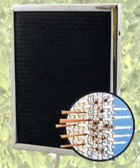
holding capacity. When particulates build up on the prefilter, air flow causes them to break off and be swept into the ACCUMULATOR CHAMBER, where turbulence and electrostatic forces cause agglomeration into even larger particulates. These agglomerated particulates are too large to pass through the second panel (afterfilter). Finally, the afterfilter attracts and holds the smaller particulates that may have escaped the prefilter, or do not respond to an electrostatic charge.
